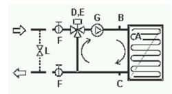
A: frost thermostat; B: air release valve; C: drain valve; D: mixing valve; E: actuator; F: ball valve; G, pump L, short-circuit bypass
