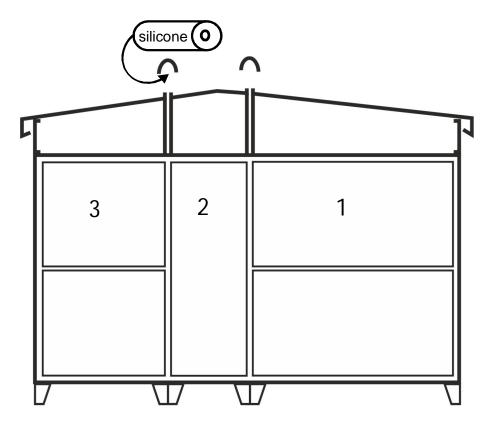
6. Seal the connections between attached U-profiles and roof plates by silicone. Seal the entire length of the connections; you will seal two connections along both ends of each U-profile.
