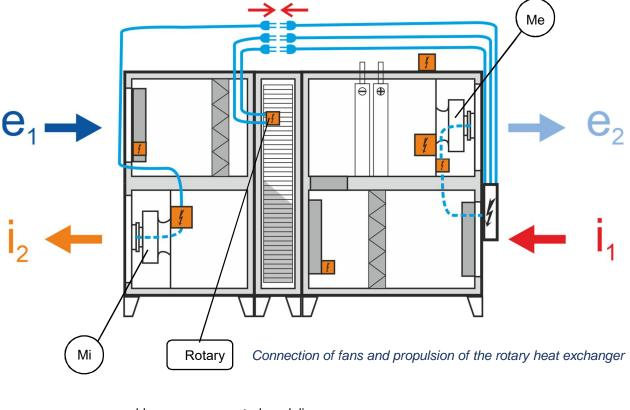
= cable comes connected on delivery = cable is to be connected
