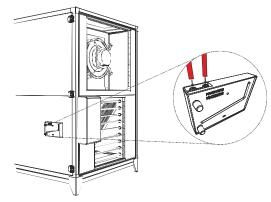
Connecting inclined manometer
