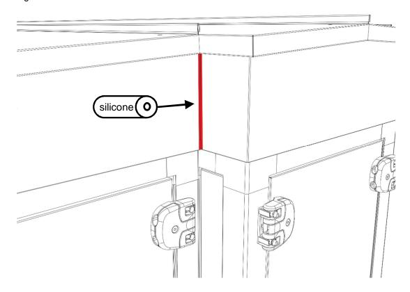
8. Seal the connection between the unit casing and the attached roof by silicone. Seal the connection all around the unit.
