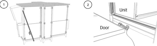
1. Securing eyelet must be tied using a tying mechanism (rope) -> the door is secured in case of wind
