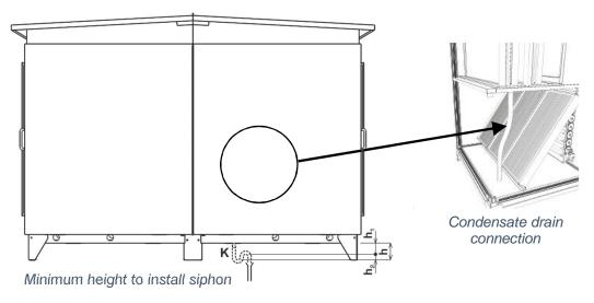
$$h_1 = \frac{\Delta p}{10} + 50 \text{ [}mm\text{]} \qquad h_2 = \frac{\Delta p}{2 \cdot 10} + 50 \text{ [}mm\text{]} \qquad h = 1,5 \frac{\Delta p}{10} + 100 \text{ [}mm\text{]}$$
